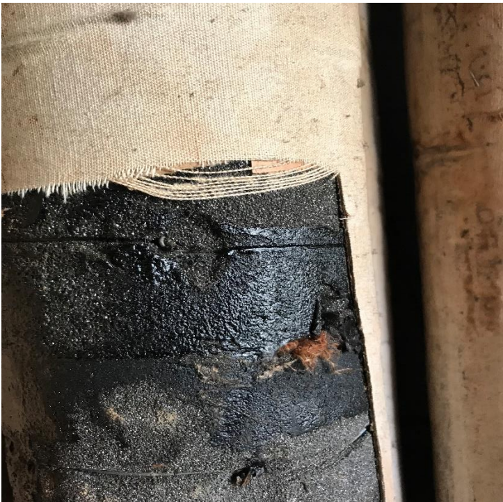
Black Mastic Under Wrap Room 0229 Sample 2-6
