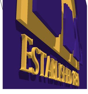
Back plate mounted directly to substrate. "Lion" plate mounted with 3/4" standoff. Mounting hardware should be of stainless or aluminum (no rust)
